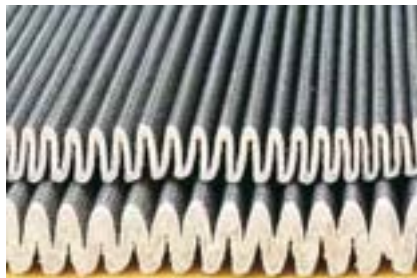
Photo above shows 'dry' Par-Gel filter media and the same media swollen with absorbed water.
