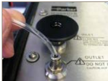
Attach OUTLET (Ø 4mm) hose
