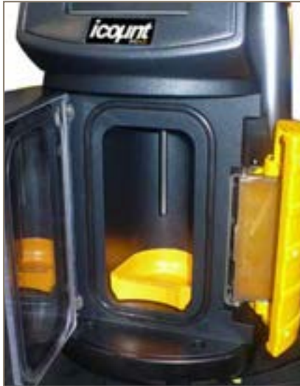
Fig 4. The IBSplus oil sampling probe automatically lowers into the bottle once the test begins.
