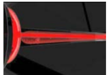
Fig 3. The shadow cast on the photo diode by contaminants in the oil creates a measurable change in the light intensity.
